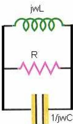
$$\frac{1}{Z} = \frac{1}{R} + \frac{1}{j\omega L} + j\omega C = \frac{j\omega L + R + (R + j\omega L)j\omega C}{j\omega RL}$$
