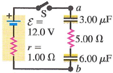
a)  $C_{\text{eq}} = \left( \frac{1}{3 \mu\text{F}} + \frac{1}{6 \mu\text{F}} \right)^{-1} = 2.00 \mu\text{F}$
