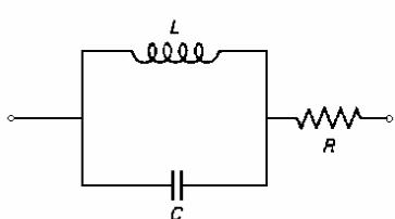
$$\frac{1}{Z_1} = \frac{1}{j\omega L} + j\omega C = \frac{1 - \omega^2 LC}{j\omega L}$$
