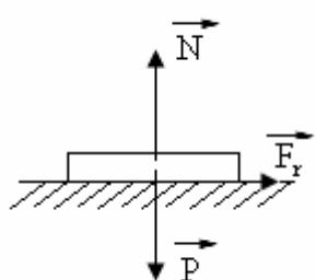
$$\begin{aligned} F_r &= N\mu = mg\mu \\ F_r &= ma \end{aligned} \quad \left. \begin{aligned} a_{\max} &= \mu g \end{aligned} \right\}$$
